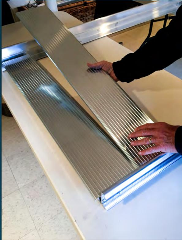
Redispan's ramp sections are truly modular. Our decking slides and interlocks into place, and is then bolted down to the side rail; versus the industry standard of using small tack welds. This unique design offers these characteristics:
